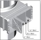
Insert weir dividers for 6" weir into two innermost tracks. 8.5" weir, use two middle tracks as shown in picture above. 16" weir, use outermost tracks.
