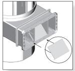
Push the weir door hinge tabs into the notches on the bottom of the weir dividers, using thumbs to hold tabs secure. Lay the door horizontal in the Skimmerfilter™ neck. \*DO NOT ATTACH THE WEIR DOOR TO THE TOP WEIR DIVIDER NOTCHES.
