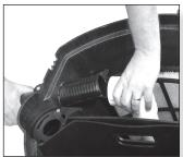
While the glue is still wet insert the Savio Aqua Flex PVC<sup>™</sup> through the side hole in the Savio Skimmerfilter. <sup>™</sup> Connect it to the pump plumbing assembly.
