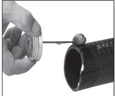
Apply the purple primer on the inside of the 90° elbow and on the outside of the Savio Aqua Flex PVC.™ Repeat, using wet weld glue.
