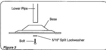
Attach Lower Pipe to Base using Bolt and Split Lockwasher. (Figure 3) FIRMLY tighten with supplied Hex Wrench.
