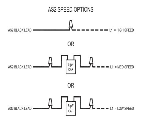
NOTE: A 2.5  $\mu\text{F}$  CAPACITOR IS ALWAYS USED ON THE 120 VAC "N" LEAD, AND IS WIRED BETWEEN THE WHITE AND BROWN LEADS OF THE MOTOR.
