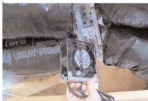
WARNING: UNPLUG FANS WHEN CHANGING DIRECTION. SEE ARROW ON BOTTOM OF FAN CARTRIDGE OR SIDE OF FAN SHROUD FOR AIR FLOW DIRECTION
