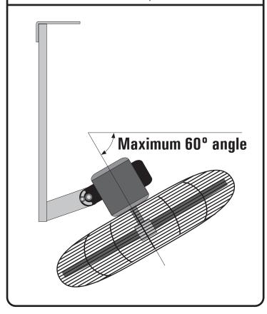
Do NOT operate the fan with the motor mounted in a vertical orientation, or at any angle larger than  $60^{\circ}$  from horizontal as shown above. Mounting this way will void the warranty.
