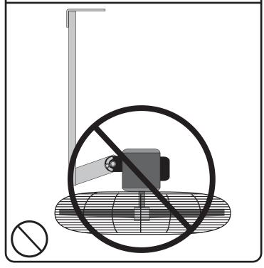
Do NOT mount fan with capacitor on the bottom. This can cause moisture to build up in the capacitor cap and short out the capacitor. Mounting the fan this way will void the warranty.
