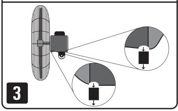
Attach fan to bracket. Insert bracket flag in between the motor flags and secure using the center holes on the motor flags with (1)  $3/8" \times 1.1/4$  hex bolt, (2) 3/8" washers and (1) 3/8" nylock nut as shown in step 4a. Using the crescent openings on the motor flags, install the (1)  $1/4" \times 1$ - hex bolt, (2) 1/4" washers and (1) 1/4" nylock nut as shown in step 4b. Adjust the fan to the desired angle and tighten hardware to secure fan angle.
