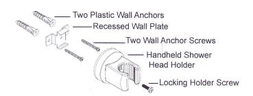
Place Recessed Wall Plate Horizontally on Wall at a Suitable Height and Mark Screw Holes. Drill 15/64" Holes for Hollow Wall Board. Insert the Plastic Wall Anchors and Tap In Flush to Wall. Screw on Recessed Plate with Screws. Attach Hand Held Shower Holder Over Recessed Wall Plate. Use Locking Holder Screw Through Hand Held Shower Bracket to Hold in Place.
