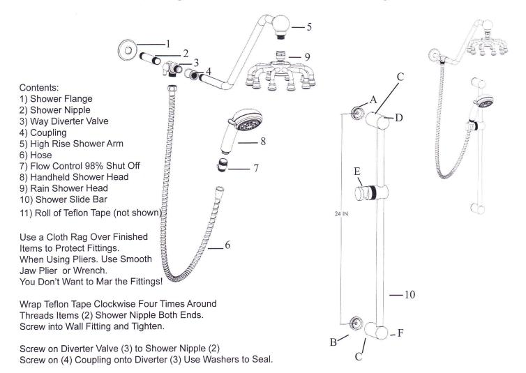
Attach Hose (6) to Diverter (3) and to (7) 98% Flow Control. Make Sure Rubber Hose Washers and Teflon Tape Are Used.
