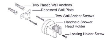
Place Recessed Wall Plate Horizontally on Wall at a Suitable Height and Mark Screw Holes. Drill 15/64" Holes for Hollow Wall Board. Insert the Plastic Wall Anchors and Tap In Flush to Wall. Screw on Recessed Plate with Screws. Attach Hand Held Shower Holder Over Recessed Wall Plate. Use Locking Holder Screw Through Hand Held Shower Bracket to Hold in Place.
