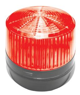
Model OE-STROBERPR is a high output, rainproof strobe suitable for both indoor and outdoor applications. Strobe life expectancy is 50,000 hours, up to 250 times that of comparable models. Mounts on bell box or other enclosure (including W Box model OE-STSTSIREN) or directly to wood or other surface. Two bolts, two nuts and two wood screws are provided. An adhesive mounting gasket is provided to enhance rainproofing. A rubber ring seals the lens with the base.
