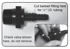
Barbed check valve is designed to be used with <sup>1</sup>/<sub>2</sub>" and <sup>3</sup>/<sub>8</sub>" tubing.
