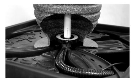
• Slide the light ring over the standpipe so that the LEDs are facing upward into the fountain. Install the ¾" insert x ¾" socket elbow on the bottom of the standpipe. Do not use glue when making this connection so that the fountain and light ring can be easily removed for cleaning or winterization.
