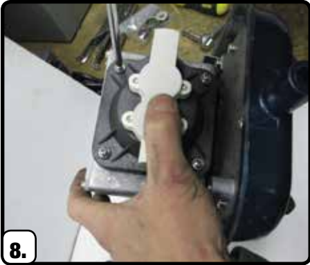
8. Re-install assembly parts onto compressor
