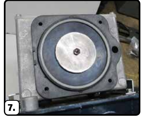
7. Place metal retainer plate on bolt and thread nut on
