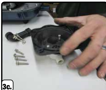
3c. Remove and replace black flapper valves
