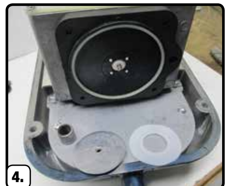
4. Unthread the \frac{9}{32} " nut and remove the metal retainer plate
