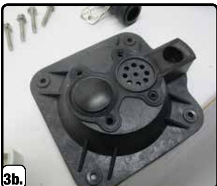
3b. Remove and replace black flapper valves
