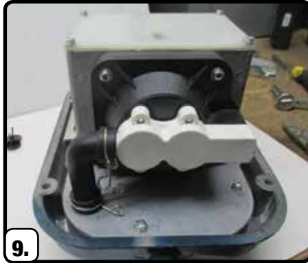
9. Tighten four screws on assembly and install black hose and clamps
