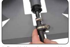
6. Fit padded hose clamp over tubing. (Use 17.5mm clamp for 3/8" tubing or 25.5mm clamp for 1/2" and 5/8" tubing)
