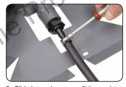
5. Slide hose clamp over fitting and fasten with regular screwdriver or nut driver.
