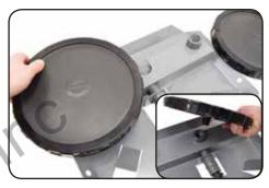
3. Screw diffuser(s) onto 3/4" FPT on top of unit. Snug fitting by hand. Do not over tighten.
