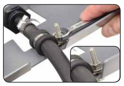
7. Use washer on both sides of base. Insert 10mm bolt from bottom side and tighten nut to clamp down tubing and provide strain relief.
