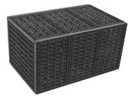
**9.**To complete the assembly rotate the EcoBlox so that the bottom panel is flat on the ground and the top panel is facing up. In this position the top panel is supported by the sides as well as the center support panels. EcoBlox should always be installed in this position. Improper installation would reduce the structural integrity of the unit and may cause the EcoBlox to fail.
