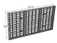
**2.** Next locate the  $14 \frac{1}{2}$ " side of one(1) of the four(4) small support panels. Insert the slide lock tabs of the  $14 \frac{1}{2}$ " side into the receiving channel at one end of the bottom panel. Holding the bottom panel in one hand push down on the support panel until it 'clicks' into position. The support panel should be centered on bottom panel.
