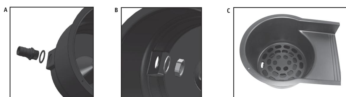
A. Place an O-ring on the hose fitting threads and insert into the back of the filter.
