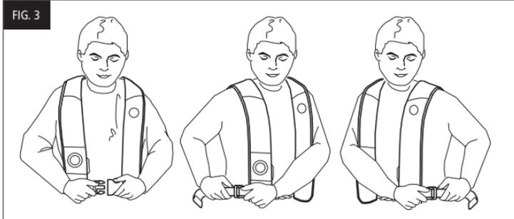
It is important that your inflatable PFD is properly adjusted to fit your body shape. An incorrect fit could result in poor performance. All belts and straps are already threaded correctly and only need to be adjusted to a tight personal fit.
