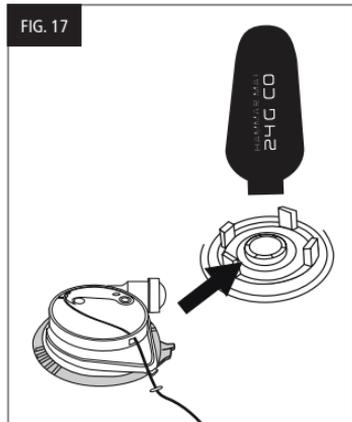
6. Check that the new inflator body indicator is green. Insert the black inflator body and cylinder into the bladder (Fig. 16). Align the cylinder with the outline printed on the bladder (Fig. 17). Ensure that the inflator body is evenly contacting the sealing ring.
