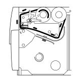
Attach the ribbon leader to the empty ribbon core using the adhesive strip on the leader edge. Turn the ribbon rewind hub clockwise until the ribbon runs smoothly through the printhead mechanism.
