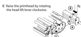
Release the lower media guide. Loosen the Unroll several inches of media and route it edge guide and slide it in to the edge of the media. Tighten the edge guide in place.
