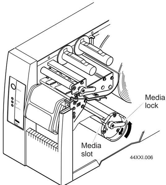
To have the media rolled onto an empty core, place the core onto the takeup hub, turn the media lock clockwise to lock the core into place, and tape the end of the media to the core.
