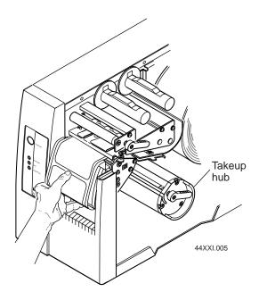
6. To have the media rolled onto the takeup hub, place the end of the media in the media slot and turn the media lock clockwise to lock the media into place.
