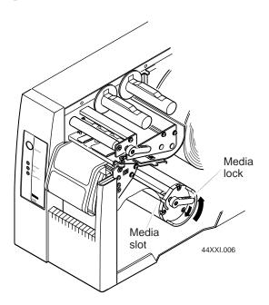
To have the media rolled onto an empty core, place the core onto the takeup hub, turn the media lock clockwise to lock the core into place, and tape the end of the media to the core.
