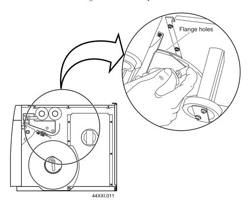
11. Reload the media, route the media below the self-strip roller, insert it into the media slot, and lock the media into place with the media lock.
