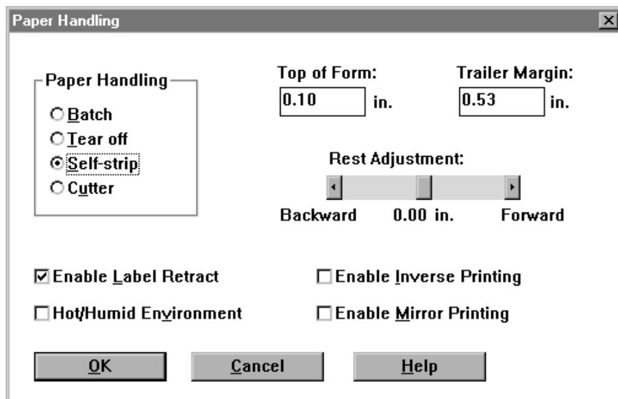
4. If you work in a hot or humid environment (temperature at or above 104°F [40°C] and humidity at or above 90 percent), select the Hot/Humid Environment box.
