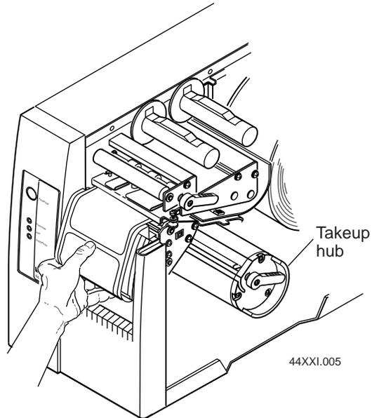
6. To have the media rolled onto the takeup hub, place the end of the media in the media slot and turn the media lock clockwise to lock the media into place.
