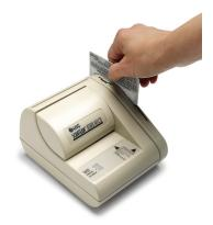
In addition to reading checks, the ST8300/ST8310 has an optional triple track magnetic stripe reader.
