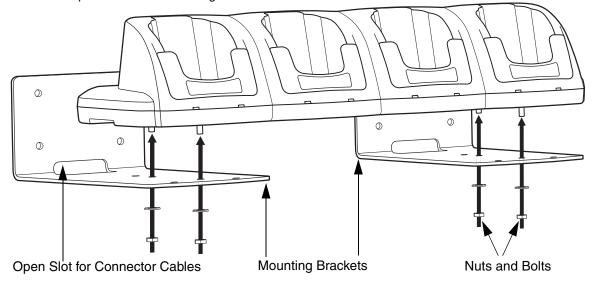
3. Using the nuts and bolts, secure the mounting brackets to the bottom panel.
