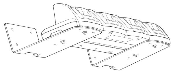
4. Secure the mounting brackets to an appropriate horizontal surface.
