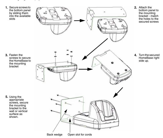
The back wedge of the mounting bracket contains an open slot for the power and communications cables. There is an extra space between this slot and the rear panel of the HomeBase to allow easy access to the power and communications ports. For more details on both ports, see Rear Panel on page 10-4.
