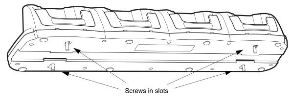
2. Attach the bottom panel to the two mounting brackets.
