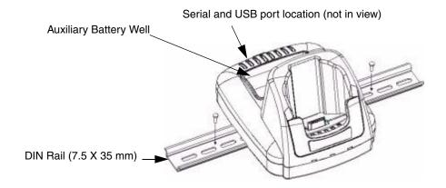
To mount the HomeBase, you slide the DIN rail slot along the bottom panel and secure it. Then, using the appropriate nuts and bolts, secure the DIN rail to the desk or flat surface.
