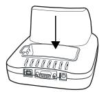
The HomeBase features an auxiliary battery well. Insert a spare battery pack into this well and the battery charges in four hours. The auxiliary battery well charges batteries independently of the terminal well.
