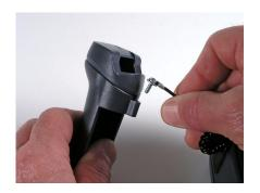
2. Peel backing from metal plate on coiled tether and affix metal plate to back of 2020 base.
