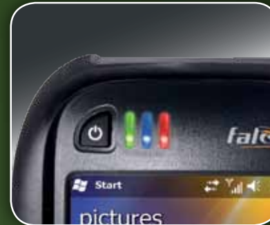
Status LEDs: power, scan and keyboard status
