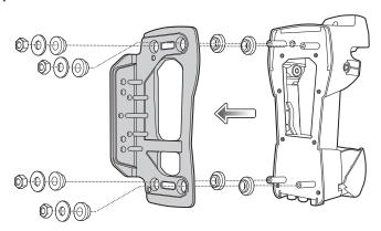
Determine if you will be installing the fork lift cradle on the right or left side of the mounting bracket.
