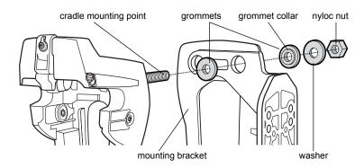
**4.** Torque the nuts to 320 in/lb  $\pm$  20 in/lb (37 kg/m  $\pm$  2.4 kg/m).
