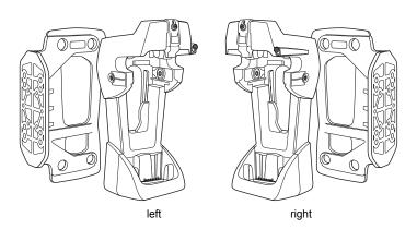
3. Install the cradle to the mounting bracket by attaching it at the four mounting points using the previously removed hardware.
