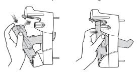
To remove the mobile computer from the fork lift cradle, lift the release button, then lift the mobile computer from the cradle. For one handed removal, use the index finger to press the release button up and then remove the mobile computer with your thumb and other fingers.
