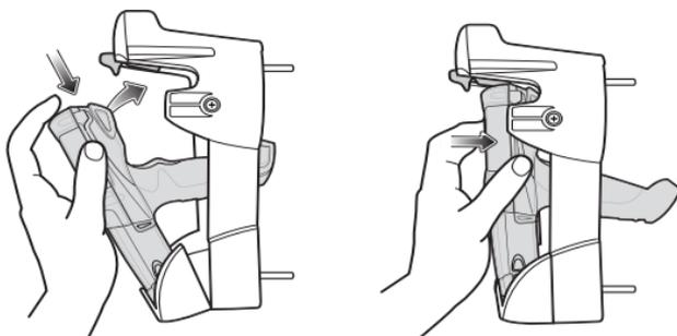
To remove the mobile computer from the fork lift cradle, lift the release button, then lift the mobile computer from the cradle. For one handed removal, use the index finger to press the release button up and then remove the mobile computer with your thumb and other fingers.
