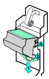
Figure 4-20: Secure the printhead cartridge
