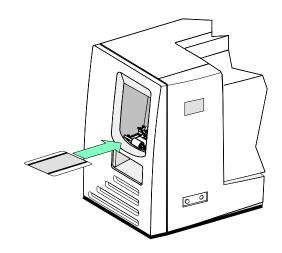
Figure 4-10: Insert the duplex/laminator cleaning card
