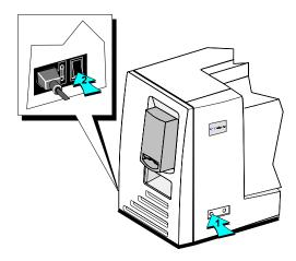
Figure 5-1: Press and hold Ready button (1) and then Press Power switch (2)
