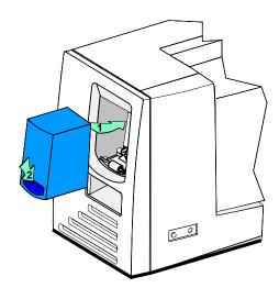
Figure 2-4: Replacing the card cartridge
