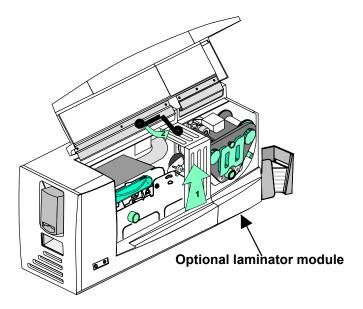
Figure 7-3: Move the top cover support down
