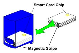
Figure 2-3: Load cards into the card cartridge
