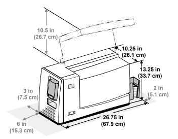
Figure 6-1: Magna Class printer without laminator, dimensions and clearance
