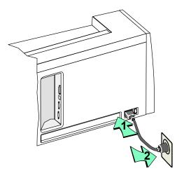
Figure 7-9: Connect the power cord
