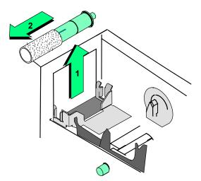
Figure 4-4: Lift the roller out of the printer
