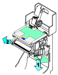
Figure 4-16: Printhead cartridge latch lever
