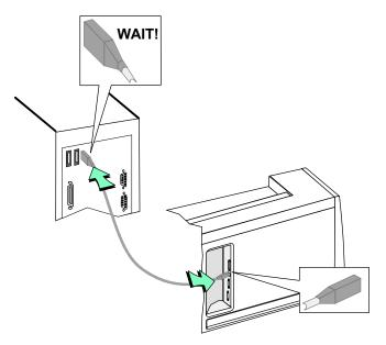
Figure 7-7: Connect the USB cable
