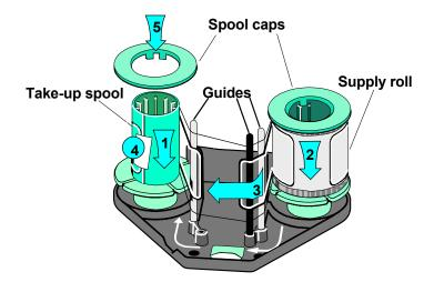
Figure 2-11: Load supply in the cartridge
