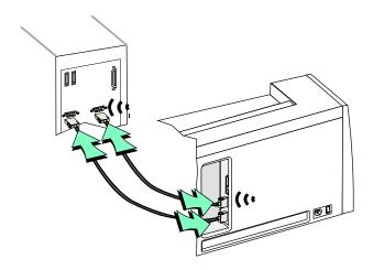
Figure 7-8: Connect the smart card serial cable
