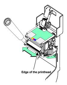
Figure 4-15: Clean the printing surface of the printhead
