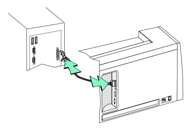
Figure 7-6: Connect the parallel port cable
