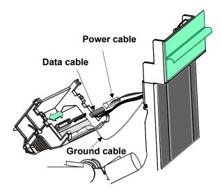
Figure 4-17: Printhead cables and connectors
