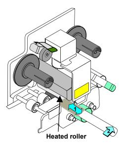
Figure 4-13: Clean the heated roller
