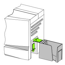
Figure 7-2: Place the card output stacker on the printer
