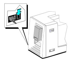
Figure 2-18: Press the power switch to power off the printer
