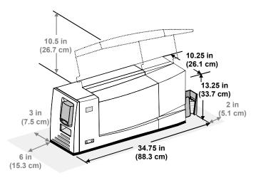
Figure 6-2: Magna Class printer with laminator, dimensions and clearance The clearance required is:
