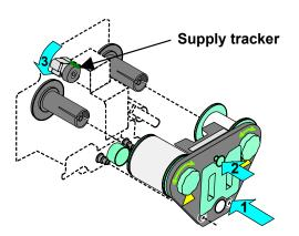
Figure 2-12: Replace the supply cartridge
