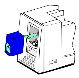
Figure 2-1: Remove the card cartridge
