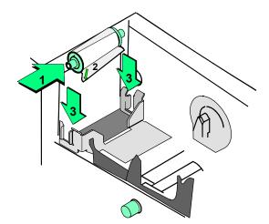
Figure 4-5: Replace the cleaning roller sleeve
