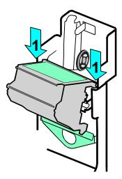
Figure 4-19: Align pins with slots on the swing arm
