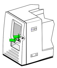
Figure 4-7: Clean the pick rollers
