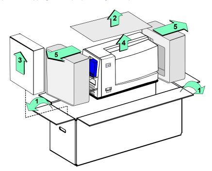
Figure 7-1: Unpack the printer
