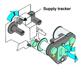
Figure 2-10: Remove the supply cartridge
