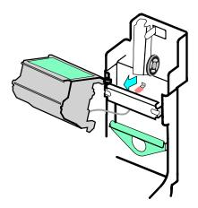
Figure 4-18: Printhead ground cable
