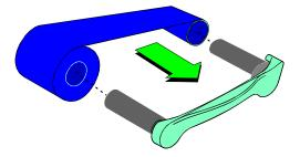
Figure 2-8: Load new print ribbon on the ribbon cartridge
