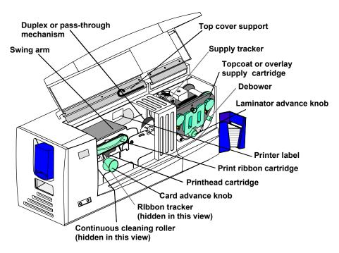
Figure 1-6: Internal parts of the Magna Class printer
