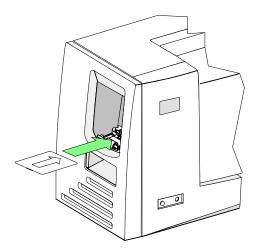
Figure 4-6: Insert the magnetic stripe cleaning card
