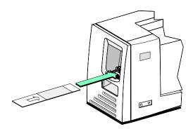
Figure 4-2: Insert the printer cleaning card
