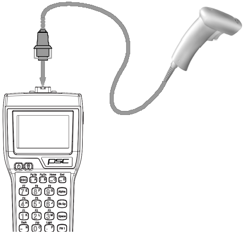
Figure 5-2: Attaching a PSC SnapShot to a Falcon 31x or 32x
