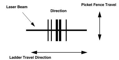
The SV unit must be programmed for the direction of travel of the codes being analyzed. If the codes are being scanned in a static condition, use the picket fence travel direction.
