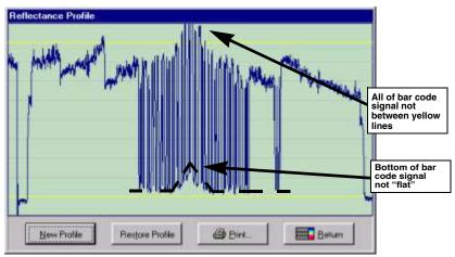
Figure 3 - Examples of Scan Profile Parameters Out of Range
