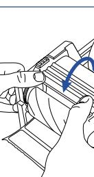
Lower the print mechanism and press down firmly to secure latches.
