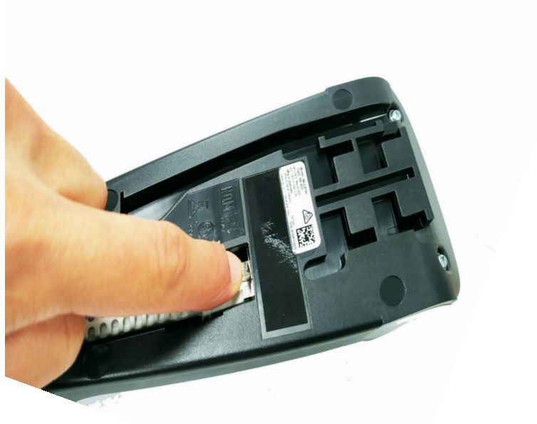
Figure 18 - Disconnecting the Cable from WLC4190
