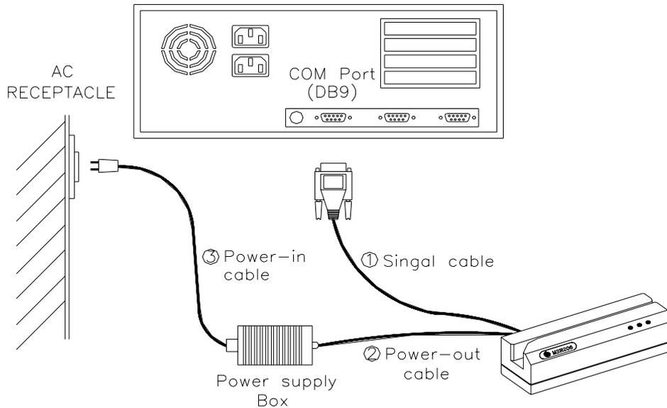
3. Connect DB9 of ① signal cable to a free serial port then connect RJ45 at the other end of the cable to MSR206
