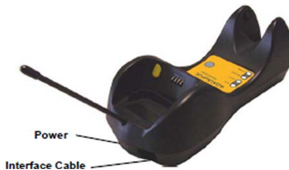
Figure 9. Disconnecting the BC-80X0 Cable
