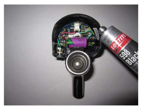
Check if the Draft Beer Counter is working properly. After, place the new battery inside the casing and apply silicone on the inside rim of the casing.
