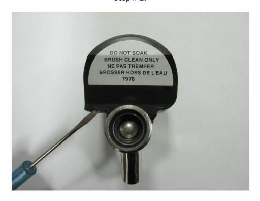
Remove the cover using a small screwdriver.
