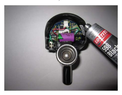
Check if the B.O.S. is working properly. After, place the new battery inside the casing and apply silicone on the inside rim of the casing.
