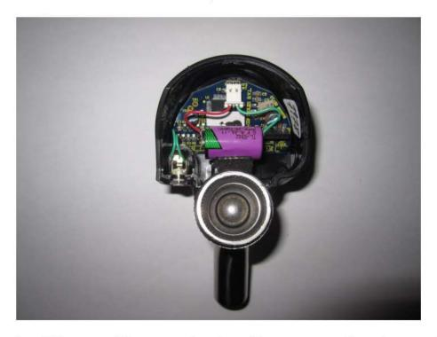
Remove the old battery. When you plug the white connector into the two pins, be sure that the RED wire is on the LEFT hand side.
