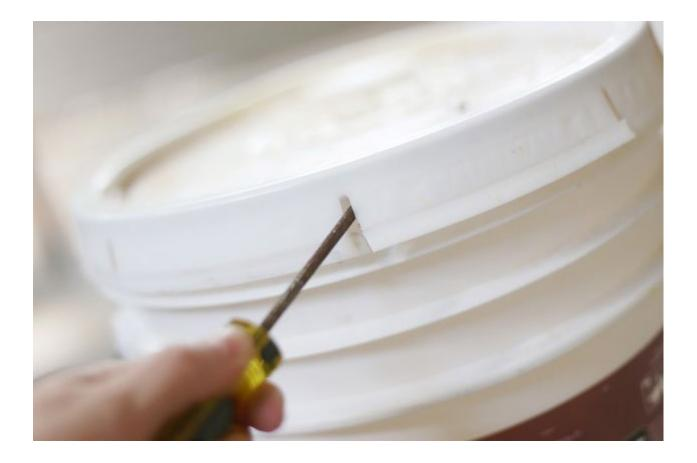
Place the screwdriver under flanges or lid rim and pry up gently. Use pliers to pull the flanges up further. Work around the bucket until the lid is loose enough to be removed with pliers or fingers. Try not to damage the edge of the bucket with the screwdriver. Levering too hard can break down the bucket edge making it difficult to replace the lid.
