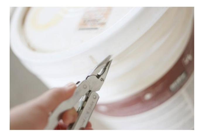
If a bucket opener is not available, use a screwdriver and pliers. It is easier to pry up the flanges if they are first cut apart at the slit. Carefully cut downward using the utility knife.
