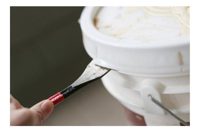
Pry upward with the handle at intervals around the lid. If the can has flanges, or tabs with a slit between them, pry at the center of a tab. Work around the lid a couple of times, if necessary, to loosen it completely. When the lid is loosened, gently pry it up and grasp the edge to remove it.
