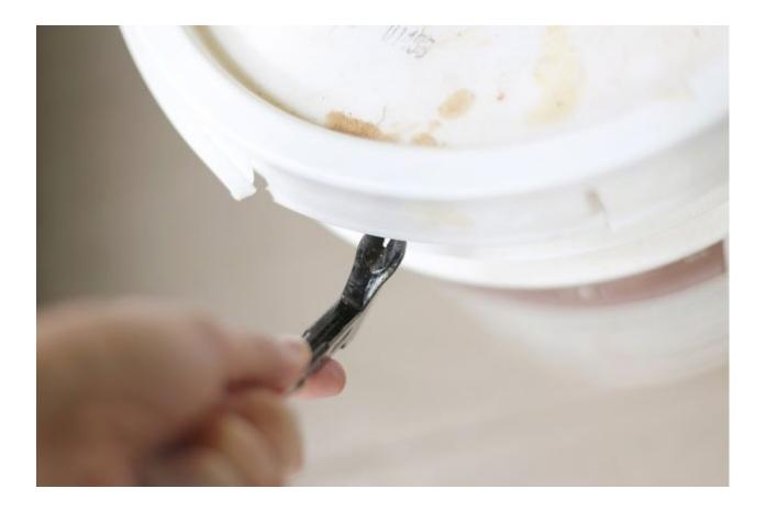
Use a paint bucket opener, if possible. It is a hard plastic tool shaped like a "C" with a handle available at paint and hardware stores. Hook the top part of the "C" over the top edge and the lower part of the "C" under the rim of the lid.
