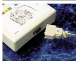
Quick disconnect allows patient to move about freely before testing begins.
