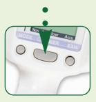
7. Press Power button to turn off monitor (automatically shuts off after 3 idle minutes)
