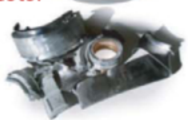
Part #K123900AS 22,640 RPM failure speed
