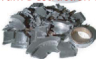
Part #K123900 36,550 RPM failure speed
