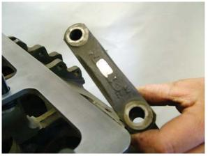
Sometimes the raised cast-in numbers on the caps need to be ground off to clear the girdle.
