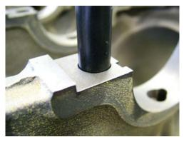
2. Use a tiny amount of mild Loc-Tite® on the studs and thread them in far enough so that when finally assembled the nut will be flush with the top of the stud.
