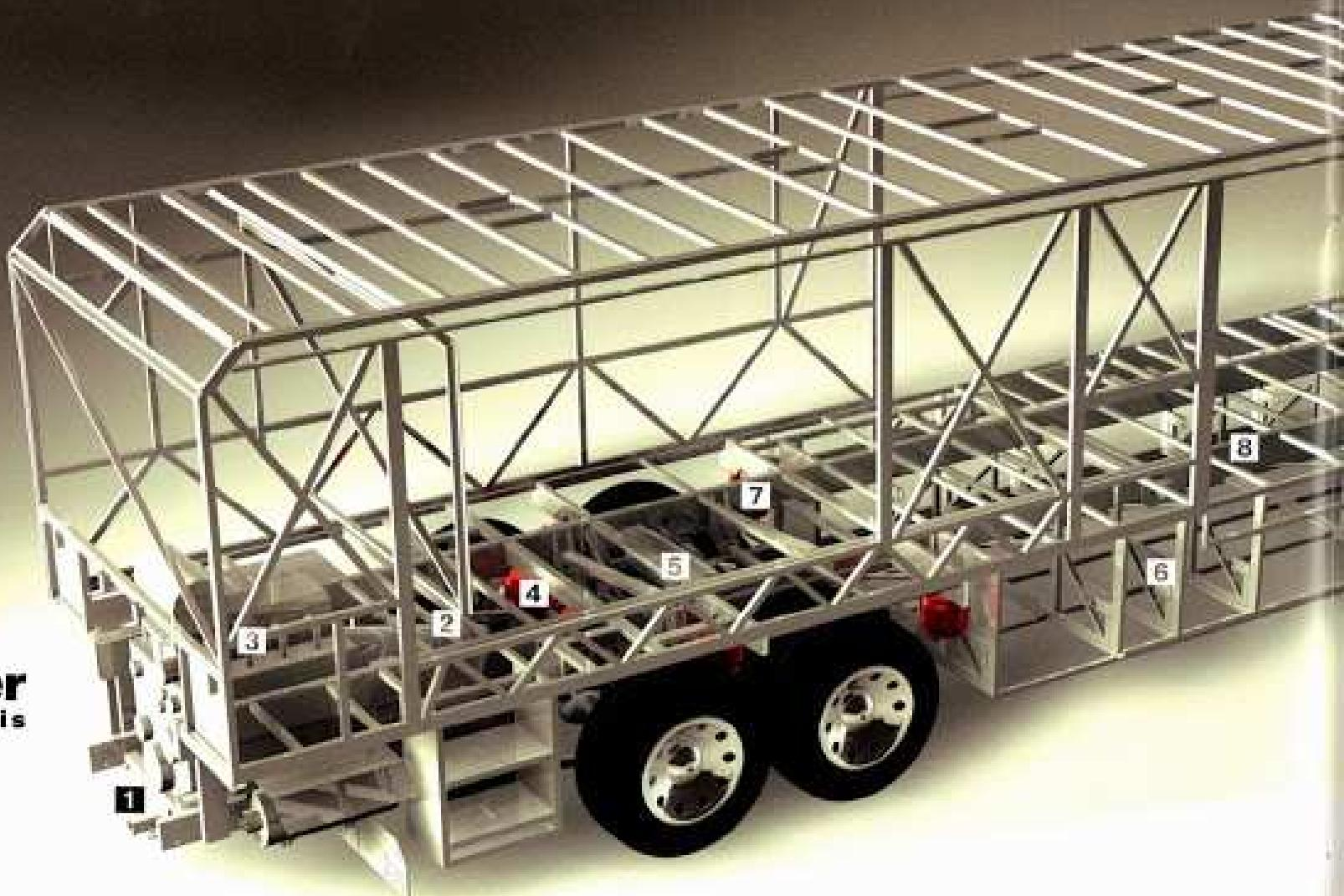
**1** 10,000 lb. hitch receiver offers powerful towing capacity with 7-way trailer plug. The coach also has a new prewire for a supplemental braking system.
