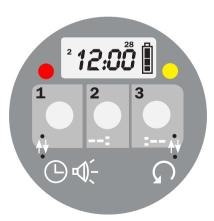
The settings of the Med-O-Wheel can only be made when its cover is removed. If necessary, see Paragraph 4.2 concerning the opening of the cover.
