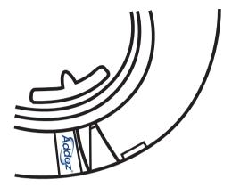
The dust cover is attached to the cassette by a locking coupling, and it can be opened and closed in only one position. If you wish to open the cover, turn it counter clockwise one notch from the zero position, so that the dispensing opening is at the position of the last compartment.
