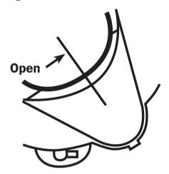
Press the black locking pin downwards and open the cover by turning it. Please note that the thread of the cover is short and corresponds to about a 30 degree turn counter clock wise ("five minutes on the clock"). See the picture.
