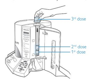
Medication is loaded on a day-by-day basis. After one day's worth of medication is loaded, the cylinders will rotate before the next day's medication is loaded.
