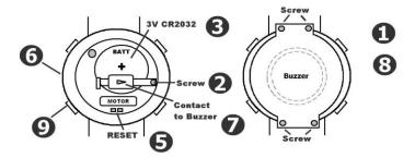
Battery: Replaceable CR2032 3V Button Cell
