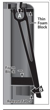
The number on each side of the hold down indicates the battery height in millimeters that hold-down can accommodate. Note that one side is labeled "28" and other side is labeled "21". The 28mm side is for use with large battery packs. If you are using very small packs, simply flip the hold-down over to the 21mm side and use it on the opposite side of the chassis.
