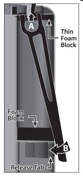
The number on each side of the hold down indicates the battery height in millimeters that hold-down can accommodate. Note that one side is labeled "28" and other side is labeled "21". The 28mm side is for use with large battery packs. If you are using very small packs, simply flip the hold-down over to the 21mm side and use it on the opposite side of the chassis.
