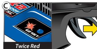
6. When the LED blinks RED TWICE. Push the throttle trigger to the full reverse and hold it there (C).
