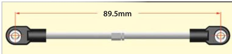
10. Connect the center drag link to one of the steering servos. Check for alignment with the holes in the second steering link. If these do not line up, make small adjustments to the length of the link until the holes line up.
