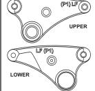
The bottom part of each rocker set is marked "This Side Down."
