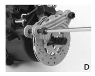
6. Thread the caliper screws into the transmission housing until there's an even amount of pressure (slight pressure) against the calipers. Once even, back each screw out one full turn. The distance between the caliper and the head of the screws should be 0.5mm. The transmission is now ready to be installed back onto the chassis (E).
