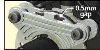
1. Use a 0.50mm feeler gauge between the brake pad insert and brake disk.
