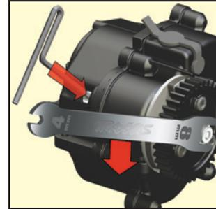
1. Limiting the engine's torque output to the wheels to prevent wheelspin on low traction surfaces and help to prevent damage to the gears in the transmission during on-throttle landings.
