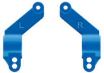
Aluminum axle carriers installed as labeled: 4° toe-in
